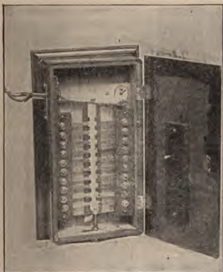
FIG. 197.—Globe selective hook switch; box open showing the slide and spring contacts, also plug in the cover.
